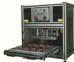
Tray out for loading (Seal area guard door removed for photography purposes)
